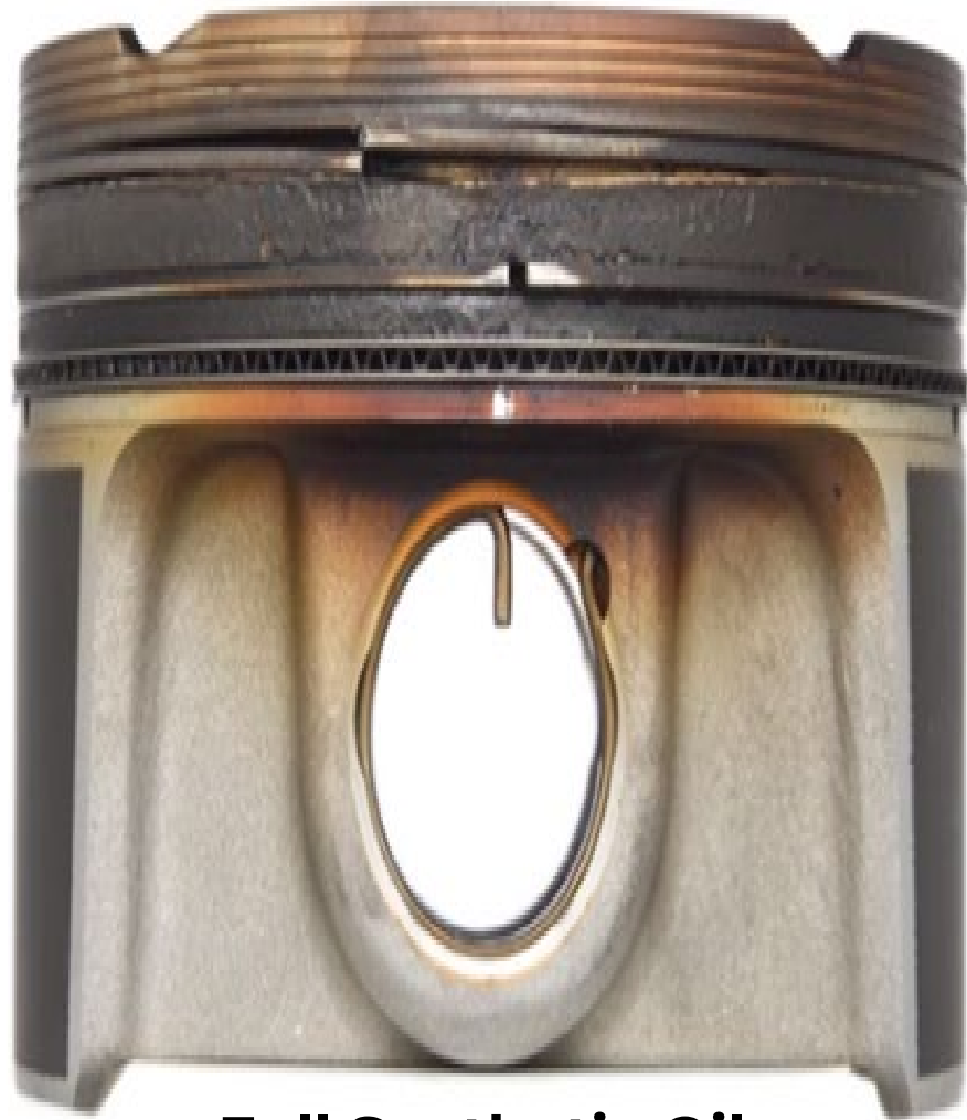
Full Synthetic Oil: FAIL ON RING groove WEAR
